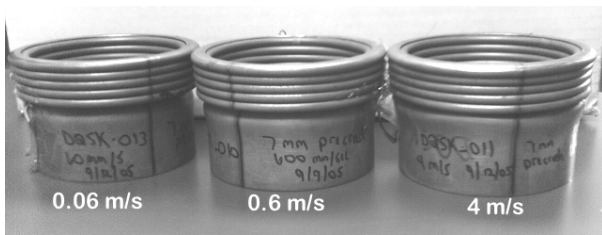
Figure 5. Specimens crushed under different velocities (Numbers in photograph denote crush speeds)
