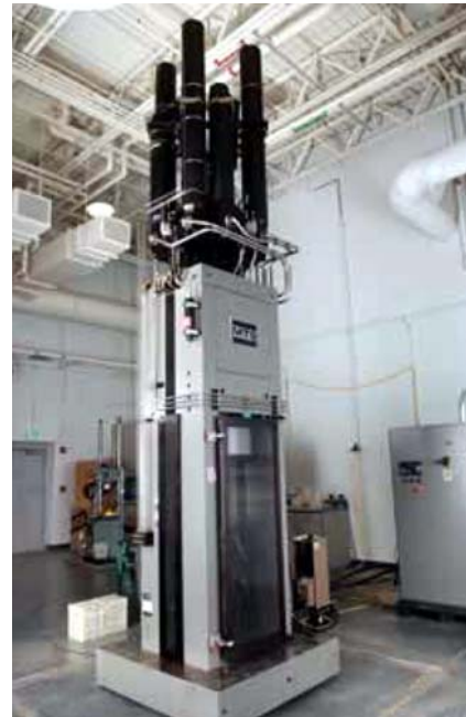
Figure 1. Test machine for automotive crashworthiness.
