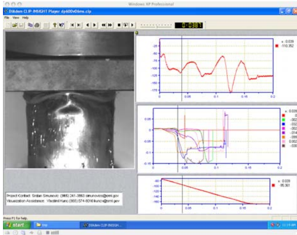
Figure 12. Tube crush data presentation
