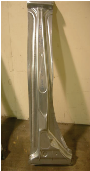
Figure 2. Body Side Center Pillar.
