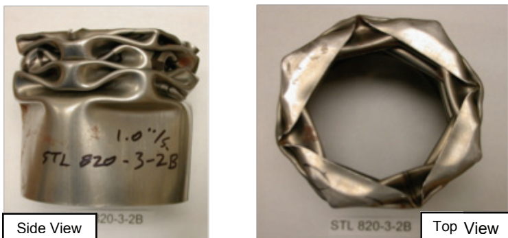
Figure 11. Baked DP780 tube tested at 25.4 mm/s
