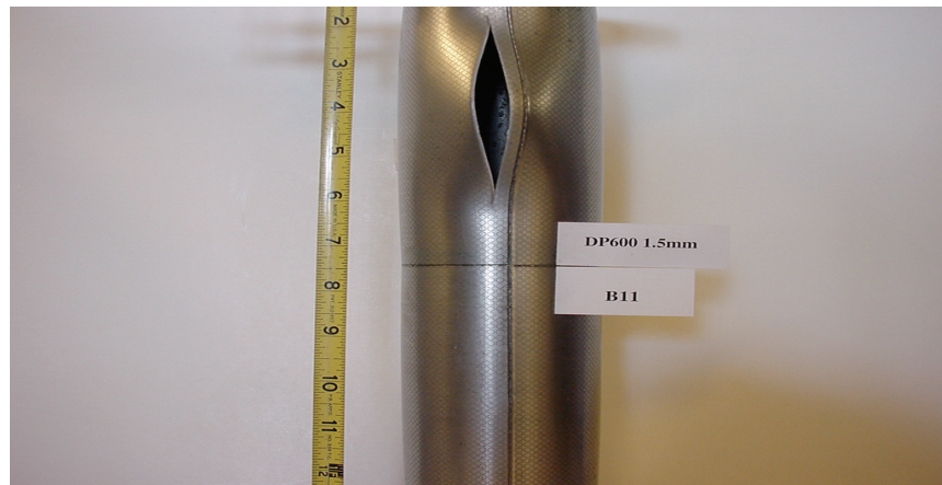
Figure 4: Example of a Burst Tube Used for Strain Measurements.
