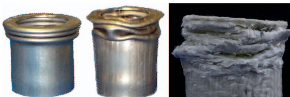
Figure 12. Concertina and diamond crush modes as seen in metallic tubes (left and center) [5] and Twintex tubes (right).
