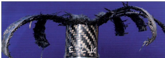
Figure 19. Unwound fronds developed in Carbon/Epoxy specimen at 4 m/s impact speed.
