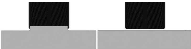
Figure 4. Showing a plug initiator (left) and flat platen (right), both specimens have a 45 Chamfer.
