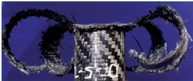
Figure 18. Separated fronds developed in Carbon/Epoxy specimen at 2 m/s impact speed.
