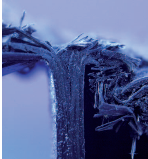
Figure 9. Fracture zone showing failed material and debris wedge in Carbon/Epoxy specimen.
