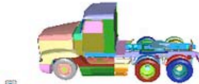
Tractor, day cabin, wheelbase 181in (file: Tractor_DayCab_181in.k)
