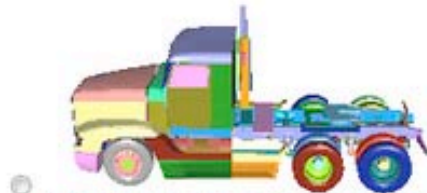
Tractor, day cabin, wheelbase 194in (file: Tractor_DayCab_194in.k)
