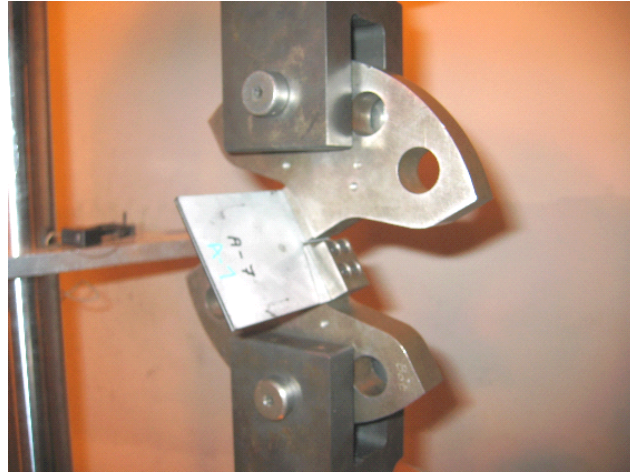
Figure 19 Set-up of mixed-mode fixture for the static test (loading angle, \theta = 30^\circ )
