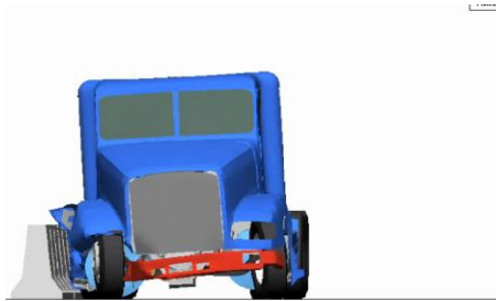
Figure 34. Photograph / Illustration. Sequential Views of FOIL Test No. 03008 and FE Simulation from a Downstream View Point.
