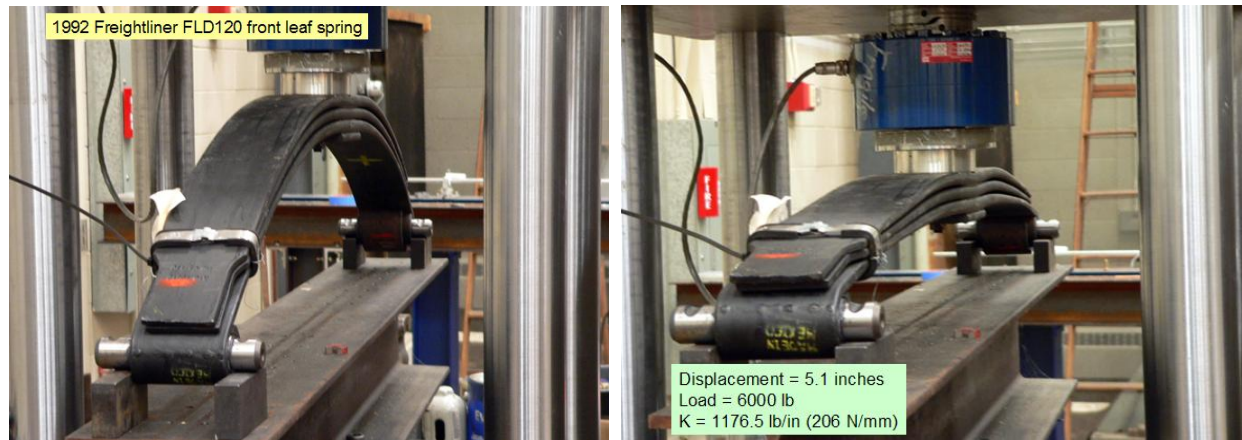
Figure 5. Photograph. Laboratory Test of a 1992 Freightliner FLD120 Leaf-spring Suspension.
