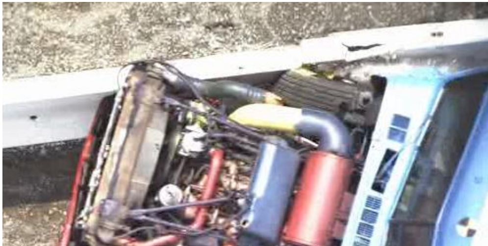
Figure 33. Photograph. Top View of FOIL Test 03008 Illustrating Barrier Movement during Impact
