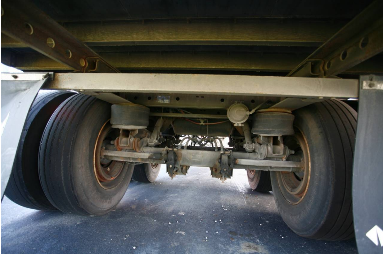
Figure 68. Photograph. Rear view of trailer vehicle frame and bogie.
