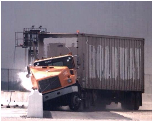
Figure 98. Photograph / Illustration. Sequential views of MwRSF Test TL5CMB-2 and FE model simulation from a downstream viewpoint.
