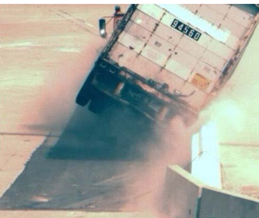
Figure 99. [CONTINUED] Photograph / Illustration. Sequential views of MwRSF Test TL5CMB-2 and FE Model simulation from an upstream viewpoint.
