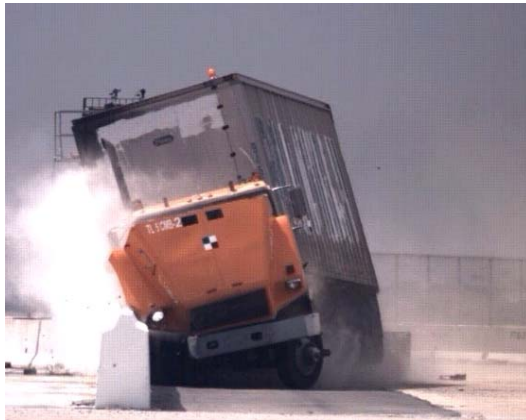
Figure 98. [CONTINUED] Photograph / Illustration. Sequential views of MwRSF Test TL5CMB-2 and FE model simulation from a downstream viewpoint.
