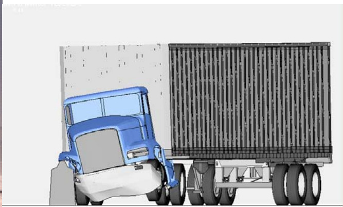
Figure 98. Photograph / Illustration. Sequential views of MwRSF Test TL5CMB-2 and FE model simulation from a downstream viewpoint.
