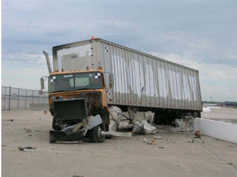
Figure 125. Photograph. Post test view of test vehicle illustrating excessive damage after secondary impact.
