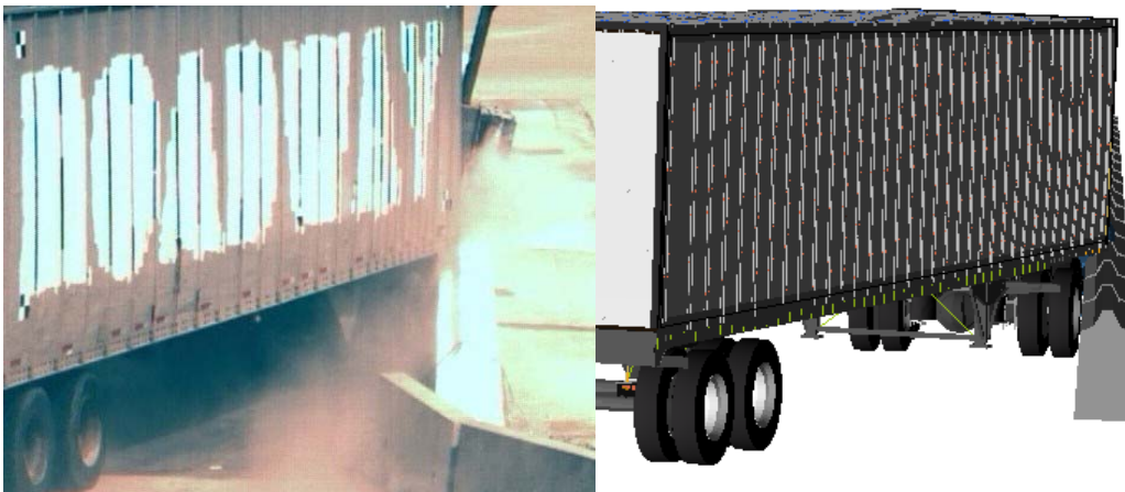
Figure 99. Photograph / Illustration. Sequential views of MwRSF Test TL5CMB-2 and FE model simulation from an upstream viewpoint.
