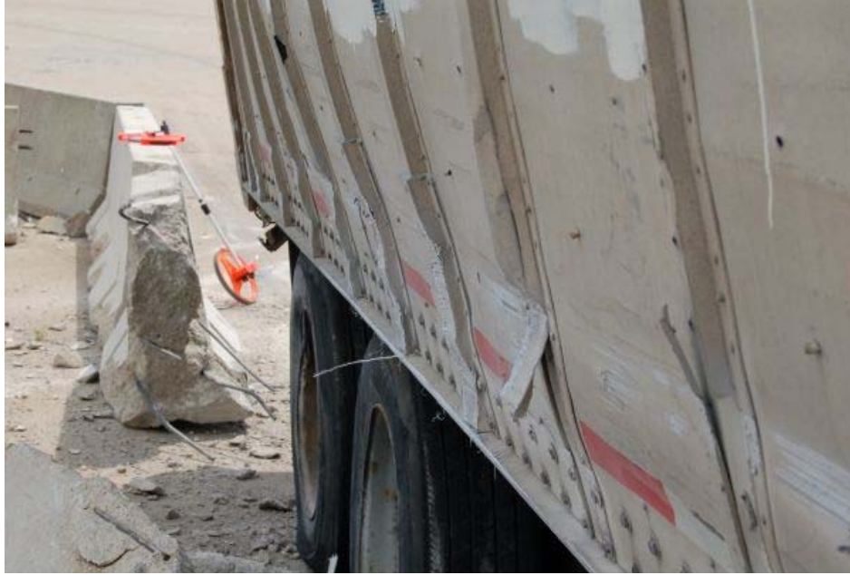
Figure 126. Photograph. Post test view of the trailer showing damage to sidewall and external ribs.
