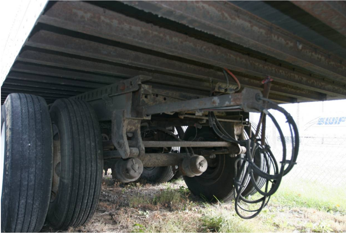
Figure 66. Photograph. Front view of trailer vehicle frame and bogie.
