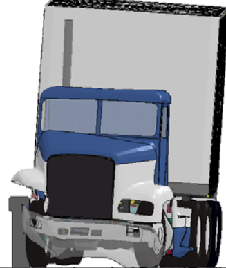
Figure 76. [CONTINUED] Photograph / Illustration. Sequential views of TTI Test 7069-13 and FE model simulation from a downstream viewpoint
