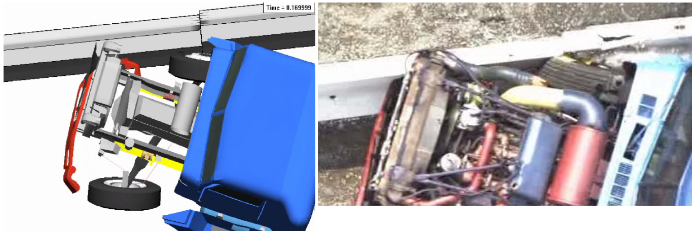
Figure 122. Illustration / Photo. Initial tire impact interaction with barrier
