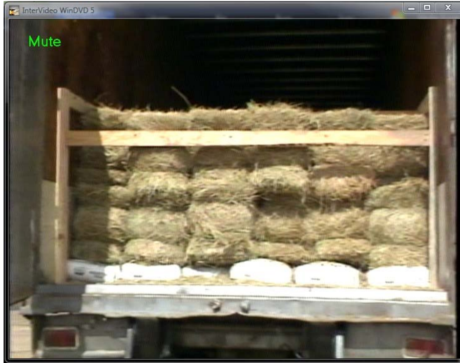
Figure 74. Photo. Trailer ballast for TTI test 7069-10
