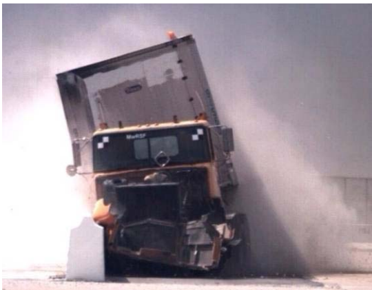
Figure 43. [CONTINUED] Photograph / Illustration. Sequential views of MwRSF Test TL5CMB-2 and FE model simulation from a downstream viewpoint
