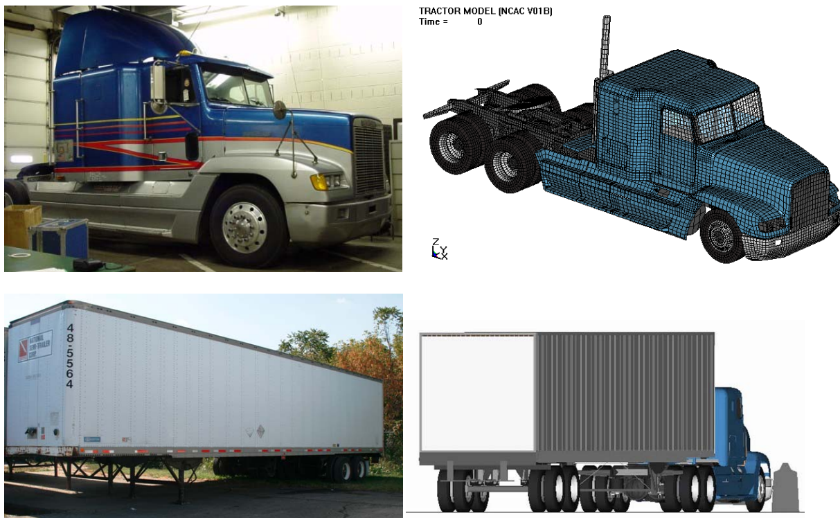
Figure D-1. Photograph / Illustration. Views of FLD 120 Tractor and 48-foot Stoughton semitrailer vehicles and FE corresponding models
