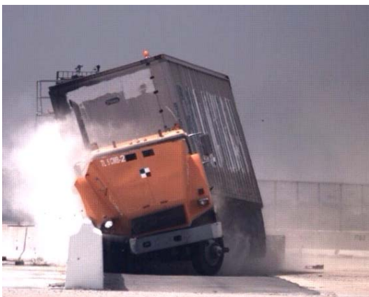
Figure 43. [CONTINUED] Photograph / Illustration. Sequential views of MwRSF Test TL5CMB-2 and FE model simulation from a downstream viewpoint
