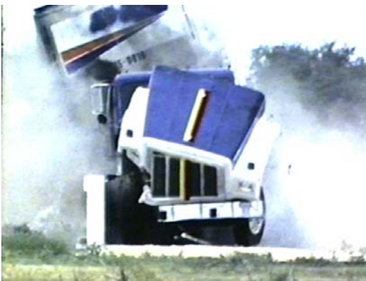
Figure 76. [CONTINUED] Photograph / Illustration. Sequential views of TTI Test 7069-13 and FE model simulation from a downstream viewpoint
