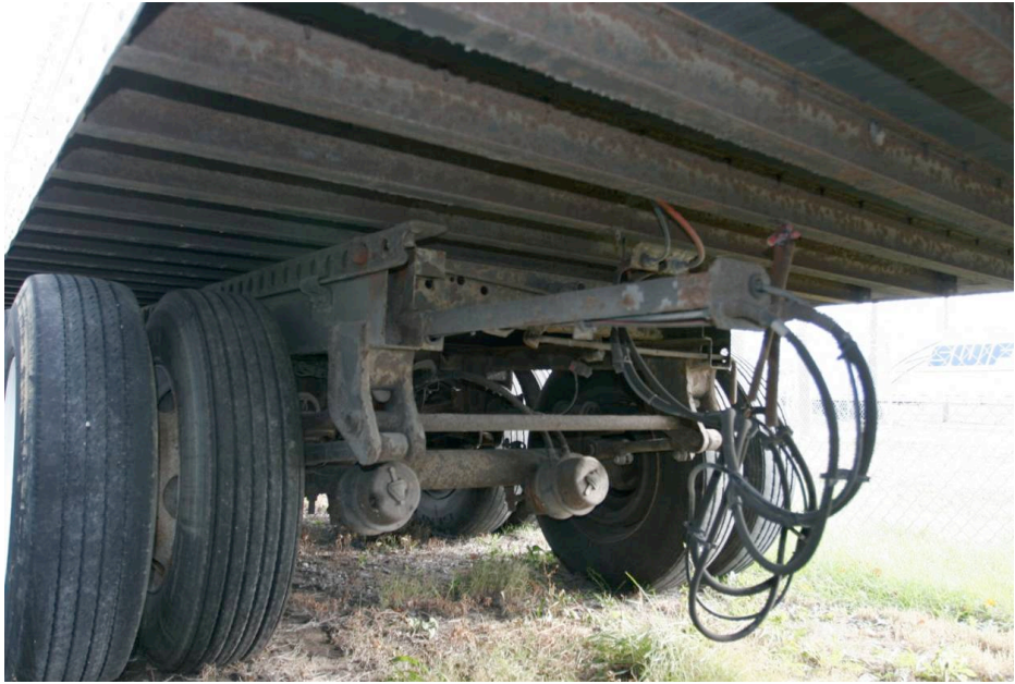
Figure 16. Photograph. Front view of trailer vehicle frame and bogie
