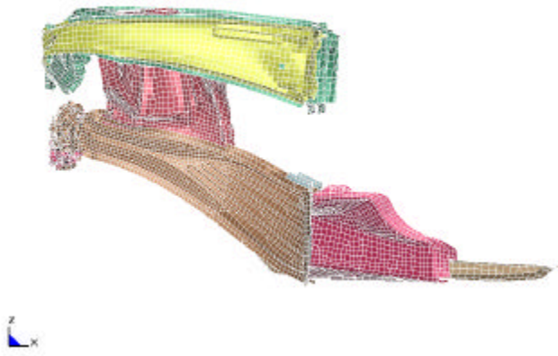
Figure 15. Front Rails – As-Formed Properties.
